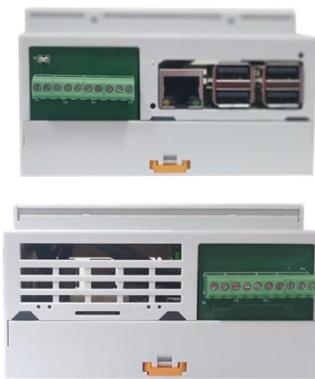
DIN RAIL Mounted I/O Module (Ref No. 8900-07)
