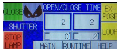
601-series touchscreen power supply automatic shutter control screen
